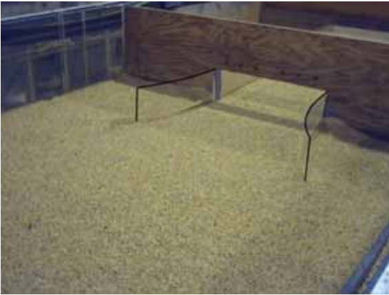
Figure 33. Photo. Elongated, streamlined wingwalls before scour.
