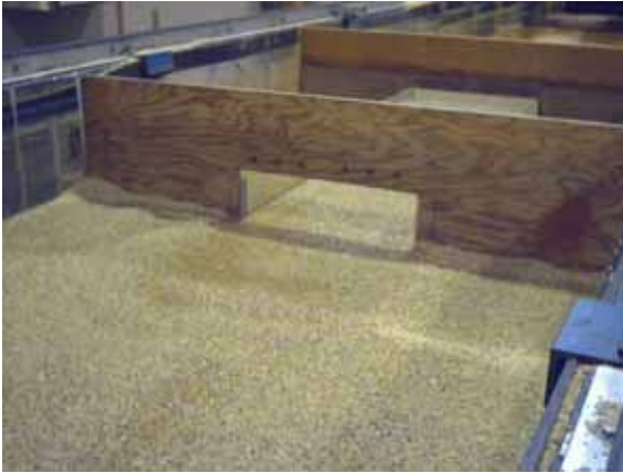
Figure 31. Photo. Truncated, circular wingwalls before scour.
