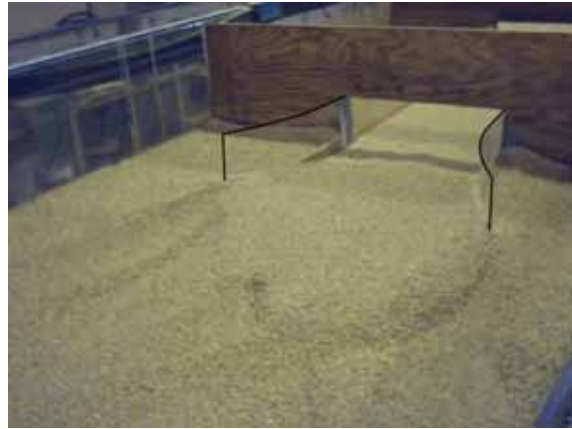
Figure 34. Photo. Elongated, streamlined wingwalls after scour.
