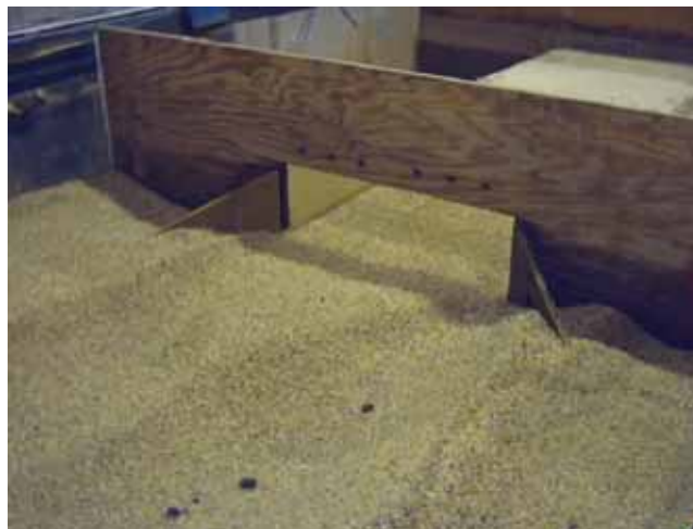
Figure 40. Photo. 45-degree wingwalls after scour.
