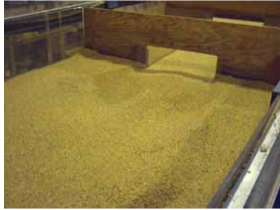
Figure 32. Photo. Truncated, circular wingwalls after scour.
