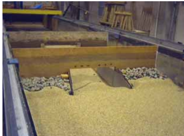
Figure 29. Photo. 8-degree inlet wingwalls after scour.
