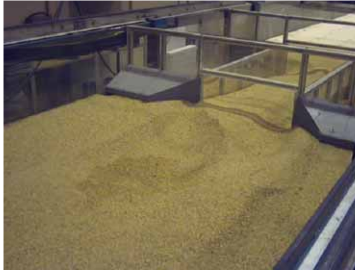
Figure 25. Photo. Outlet scour after test.
