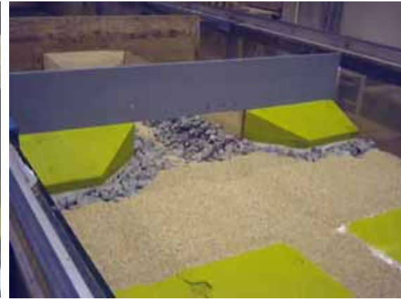
Figure 51. Photo. Shifted riprap in culvert inlet after Standard Plan test.
