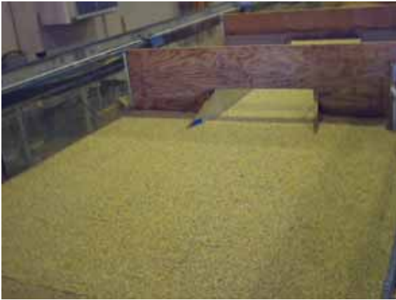
Figure 38. Photo. Wingwalls with 8-degree flare (smooth joint) before scour.
