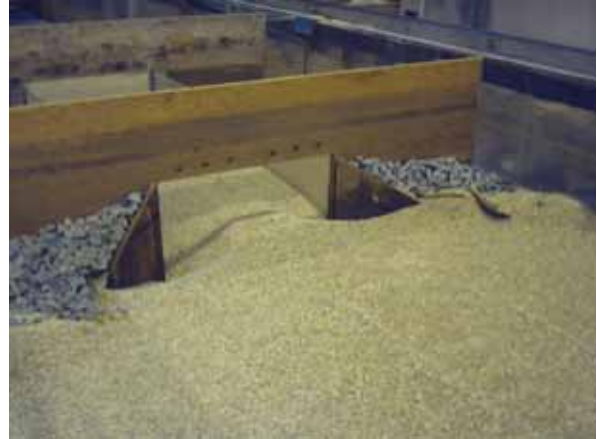
Figure 27. Photo. 45-degree inlet wingwalls after scour.
