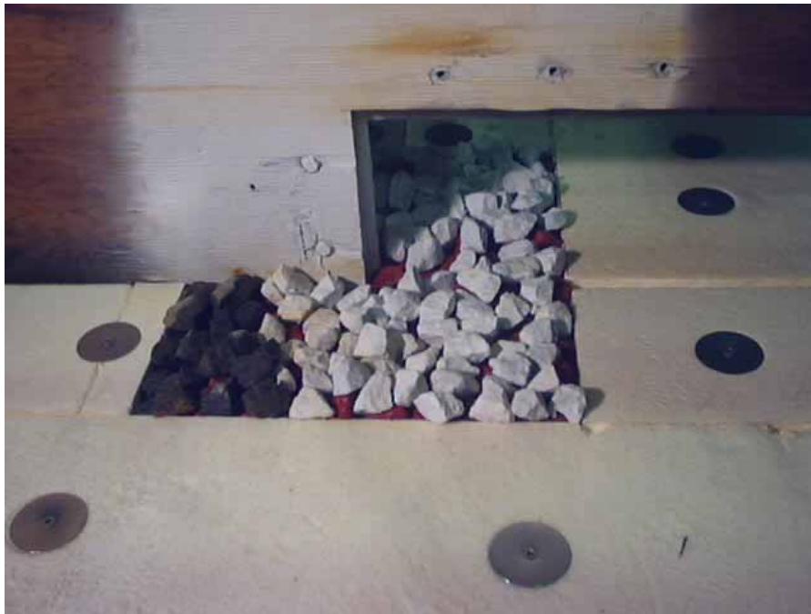
Figure 3. Photo. Riprap test for a rectangular culvert.
