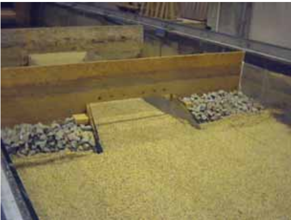
Figure 28. Photo. 8-degree inlet wingwalls before scour.
