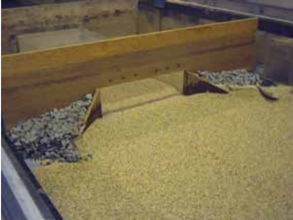
Figure 26. Photo. 45-degree inlet wingwalls before scour.
