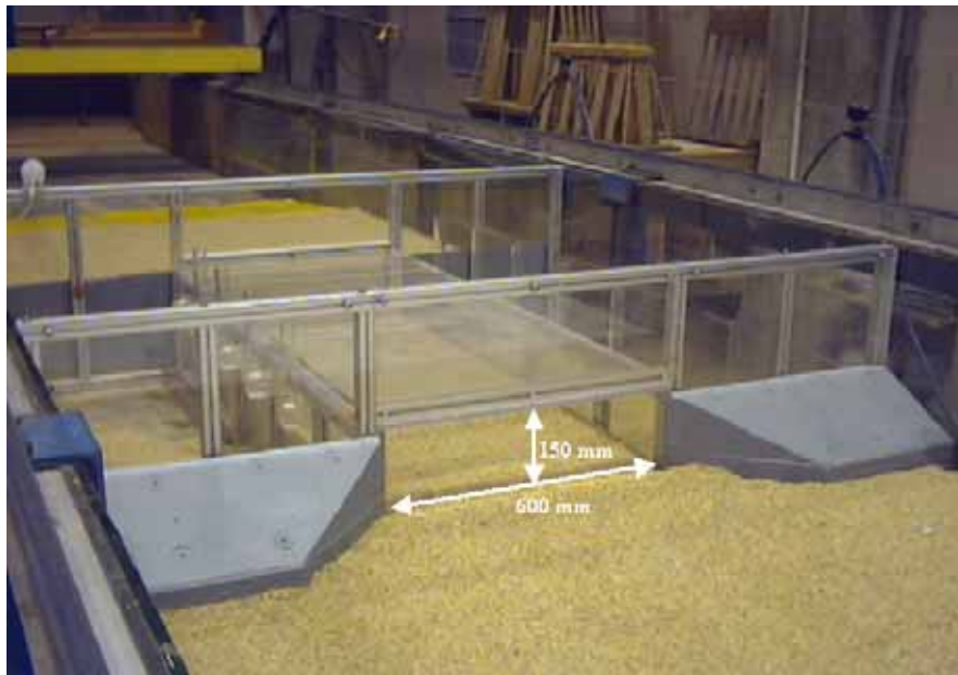
Figure 2. Photo. Rectangular culvert.
