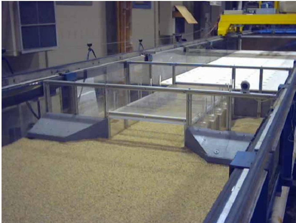
Figure 19. Photo. Outlet prior to scour test.
