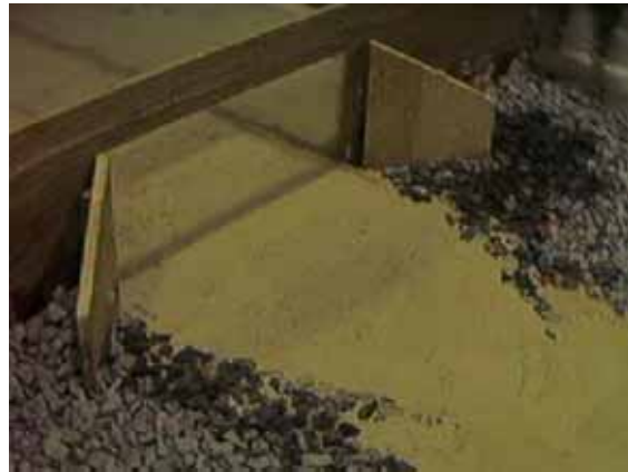
Figure 59. Photo. Cross vane installed at inlet of experimental culvert.
