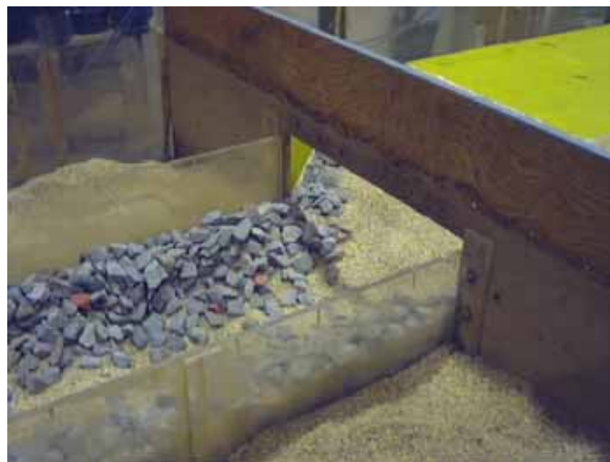
Figure 52. Photo. Shifted riprap in culvert barrel after Standard Plan test.
