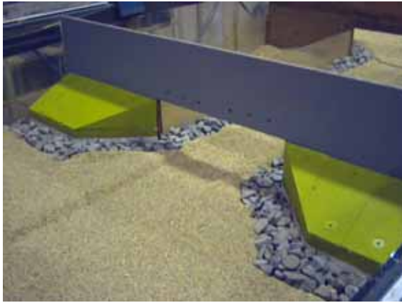
Figure 50. Photo. Culvert outlet before Standard Plan test.
