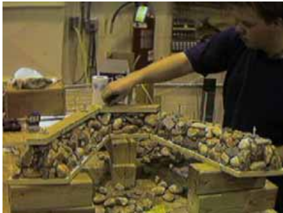
Figure 58. Photo. Fabrication of the cross vane.
